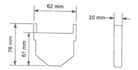
Figure 9 - Drop Connector Dimensions
