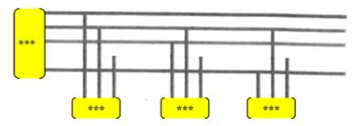
Figure 5 - Three Phase Trunk, Single Phase Drop Application
