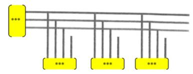
Figure 3 - Non-Rotating Phase Application
