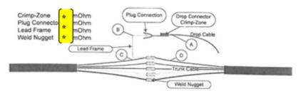
Figure 6 - Contract Resistance Schematic
