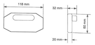
Figure 7 - Splice Box Dimensions
