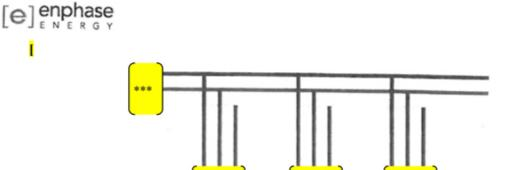
Figure 4 - Single Phase Trunk and Drop Application
